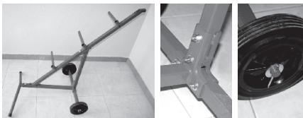
2.- With the structure secured and stable, you can assemble the rest of the parts; screw on the handle and position the hose using a little of alcohol, fit the tape bracket and secure it with the washer and nut. Position the diagonal bars and secure them with a bolt each. It is important at this point to check that the assembly is perfectly stable and that all of the nuts are tightened.
