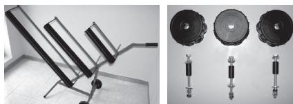
5.- The tape holders are assembled using the three extra-long bolts supplied, with two washers, and a plastic bearing, secured with two nuts each. Once fixed in their place, check they turn freely.
