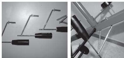
6.- The paper guides only need the three springs supplied, one per guide, to secure them in position so that they fulfil their function.
