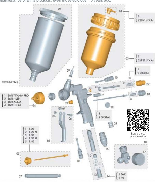
Critical parts are those that can produce a malfunction in a spray gun: Wearing parts, seals, gaskets, glands... Sagola spray guns contain **ONLY 6 CRITICAL PARTS** ( \_\_\_\_\_). Just 6 references to store and provide a 100% effective after-sales service.
